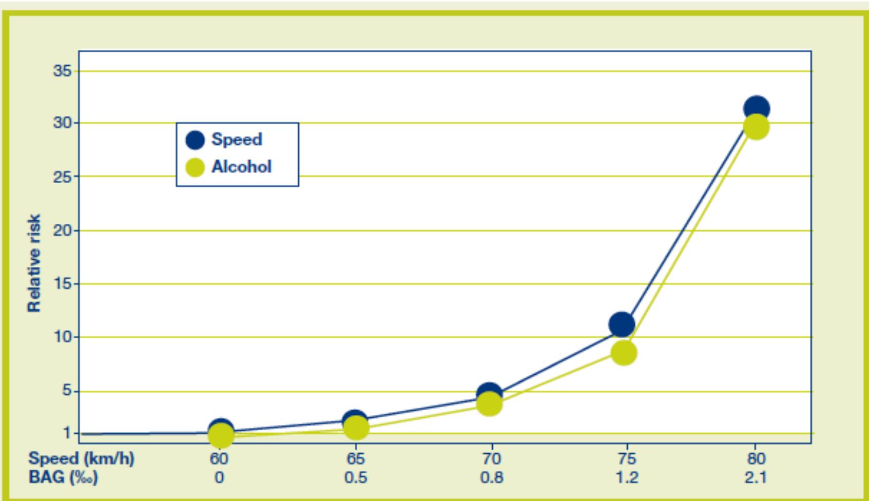
Figure 2. The relative crash risk whilst driving under the influence of alcohol and at different speeds (on Australian urban roads with a speed limit of 60 km/h). From this graph it can be concluded that driving too fast is at least as dangerous as driving under the influence of alcohol.
